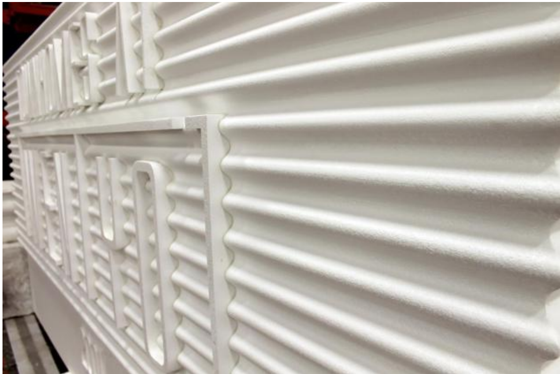
Signs By Benchmark replicated the look of corrugated metal by using hot wire cutting equipment to shape its expanded polystyrene foam.
